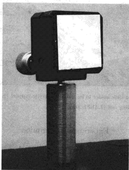
Mirror on a movable mount with two adjusting knobs and support post (LABEL B).
