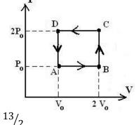
and volumes between  $V_0$  and  $2V_0$ . What is the coefficient of performance for this refrigerator? (A)  $\frac{1}{4}$  (B)  $\frac{1}{3}$  (C)  $\frac{4}{3}$  (D)  $\frac{11}{2}$  (E)  $\frac{13}{2}$
