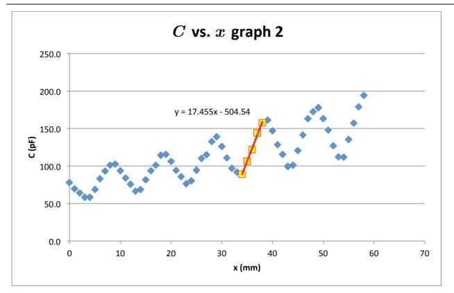
From this graph,  $m = 17.5 \text{ pF} / \text{mm} = 1.75 \times 10^{-8} \text{ F} / \text{m}$ . Using this value of m, f = 5 kHz,  $\alpha = 714 \text{ nF/s}$ , and  $\Delta f = 0.01 \text{ kHz}$ ,
