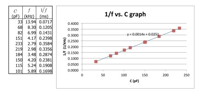
From this graph, the slope  $(1/\alpha)$  and the Y-intercept  $(C_s/\alpha)$  is equal to 0.0014 s/nF and 0.0251 ms respectively.
