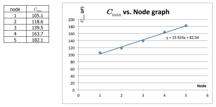
This graph is linear of which the slope is the dropped off capacitance  $\Delta C = 19.9$  pF/section.
