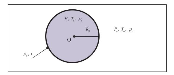
Cutting the sphere in half and using the projected area to balance the forces give
